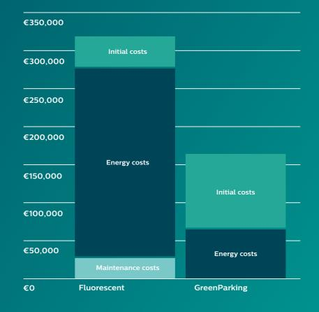
$^*$ 1x58wTL-D installation versus GreenParking system over 10 years, on 450 luminaires in typical covered parking garage at €0.12 energy price
